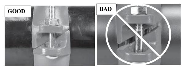
4. Visually inspect the complete system to verify all bolts are tight, coupling halves are together, and couplings are fitted properly into the tube and fitting grooves.
